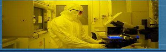
A micro-fabrication engineer working in a clean room. They have to extra caution not to bring dirt and other contaminants into the room to protect the nano-devices from possibly being ruined if a speck of dirt were to come in contact.
