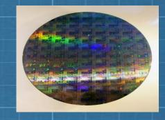
A silicon wafer is usually the base on which circuits are built on due to its ideal semiconductor properties
